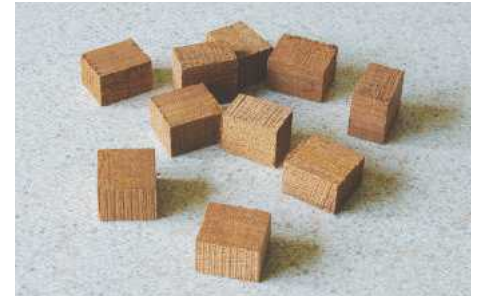
▲ Pic.9 From some 12mm-thick mahogany, cut 20 squares each with 20mm sides
